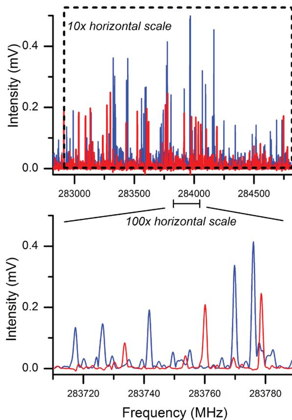
**Fig 4:** An overlay of the 2-methylimidazole (red) and the 4(5)-methylimidazole (blue) spectrum. The 100x horizontal zoom highlights the high resolution of rotational spectroscopy.
