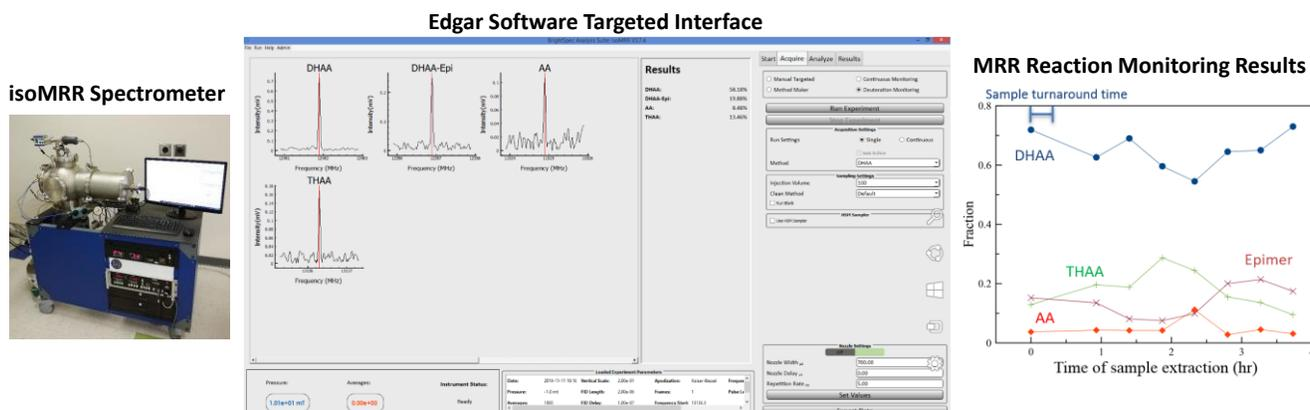
**Figure 2. Left Panel:** Picture of isoMRR instrument capable of online and at-line quantitative analysis of impurities in complex chemical mixtures including regioisomers, diastereomers, enantiomers, dehalogenation species, isotopologues, and isotopomers.
