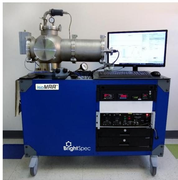
**Figure 1.** A picture of a commercial isoMRR™ unit capable of quantitative analysis of impurities in complex chemical mixtures including regioisomers, diastereomers, enantiomers, and isotopomers. Instrument is equipped with online-capable sampling manifold.
