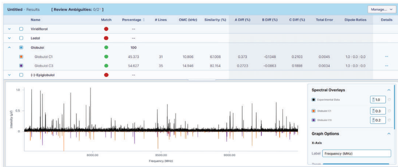
Figure 5. Spectral fitting and structure confirmation of an unknown sample using Edgar. Edgar's data analysis interface compares experimentally acquired MRR spectra from an unknown sample against a library of simulated rotational spectra for candidate structures, including viridiflorol, ledol, globulol, and epiglobulol. The results indicate a 100% match to globulol, while other stereoisomers show no valid match. Spectral overlays (bottom) illustrate the alignment between experimental data (black) and simulated globulol transitions (colored), confirming molecular identity based on unique rotational fingerprints rather than molecular formula alone.
