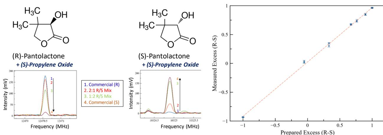
**Figure 2.** Targeted MRR method validation using prepared mixtures of commercial (R)- and (S)-pantolactones. MRR shows excellent analysis sensitivity, linearity, range, and repeatability.
