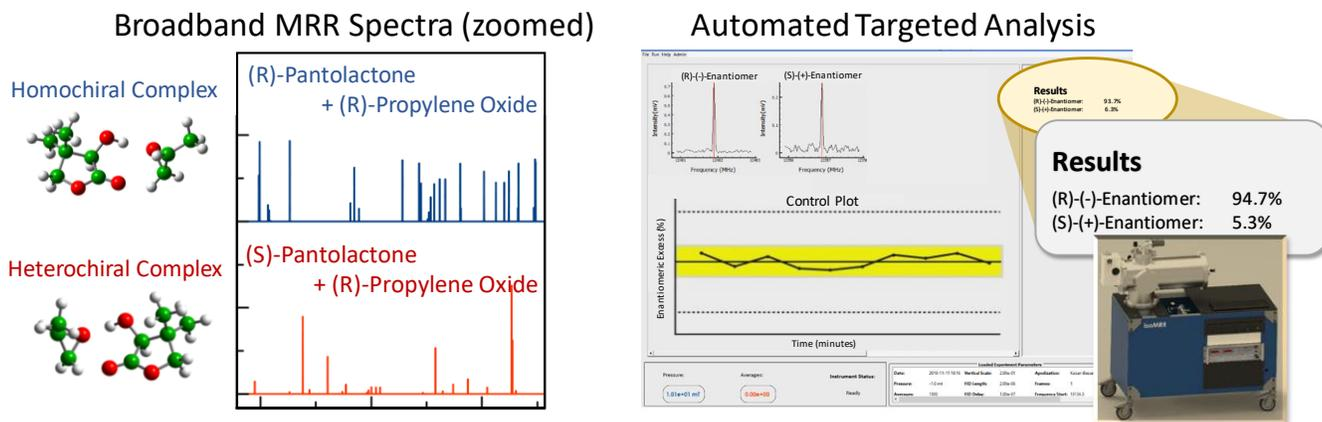
**Figure 1.** Left Panel. Broadband MRR spectra of homochiral (blue) and heterochiral (red) complexes between the analyte (pantolactone) and the low-cost gaseous chiral agent ((R)-propylene oxide). Right Panel. Example of fully automated analysis performed by a BrightSpec’s targeted isoMRR instrument. The analysis can be executed every ~10 minutes and requires no enantiopure standards or sample purification.
